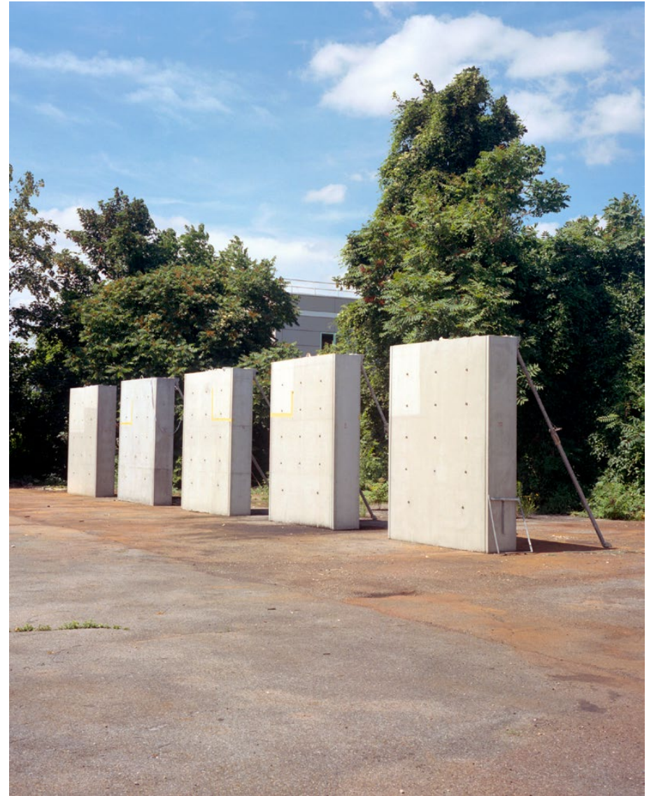
Concrete testing for Tadao Ando's Bourse de Commerce redesign, Pantin, June 2018
